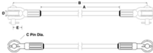
Guy Strain ; 16,000 lbs.; Clevis - Clevis - 2 Roller
