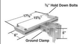
Aluminum Capacitor Rack, pole mounted, for mounting one capacitor with 15 5/8" lug spacing weighing up to 80 lbs. each. Includes two pre-spaced 3/8" hold down bolts, flat washer, lockwasher and nut per capacitor mounting position and a ground wire clamp secured with 3/8" bolt. Supplied factory assembled and ready for installation of capacitor.
