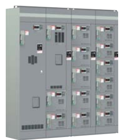
Low Voltage Model 6 Motor Control Centers 600 Volts Maximum 50 to 60 Hz Bus Ratings up to 2500 A Control Control: 120 Volts 60 Hz, 110 Volts 50 Hz
