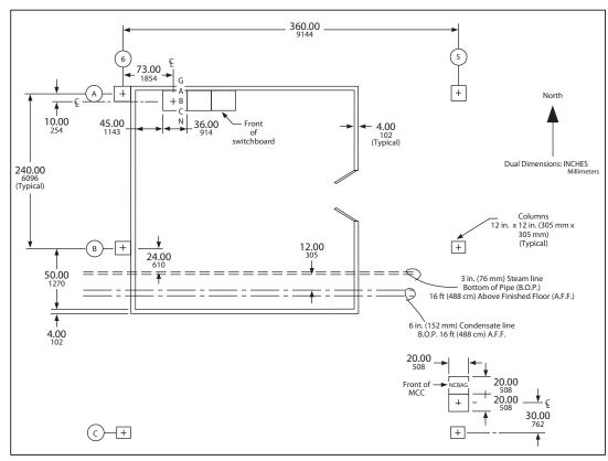
Figure 20: Plan View Switchboard, MCC, and Obstructions
