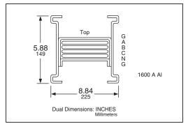
Figure 19: Physical Size of Busway Housing
