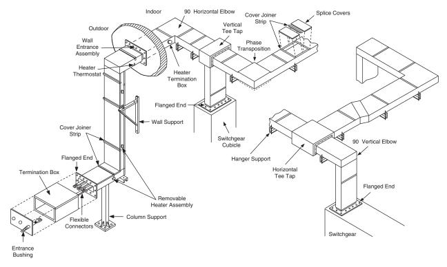
Figure 25: Typical Layout Example
