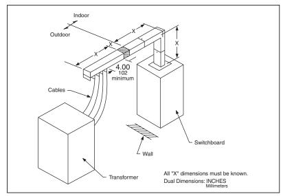
Figure 8: **Transformer Tap for One Three-Phase Transformer**
