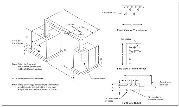
Figure 11: Information Needed for Bussed Transformer Connection (Pad Mount Type)
