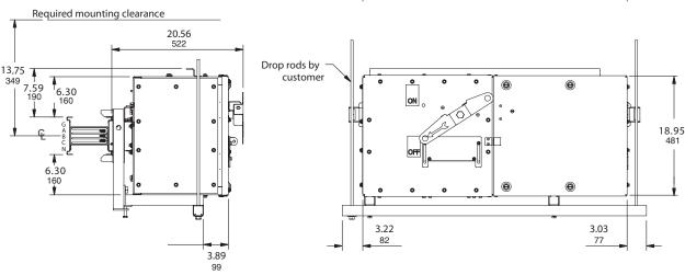
NOTE: Bolt-on units to be used only on plug-in busway with the same number of poles. Not for use on 800 A copper busway.
