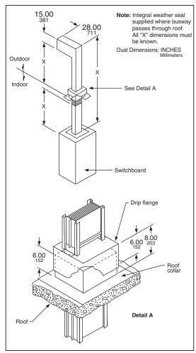
Figure 7: **Vertical Service Head** Penetrating a Roof
