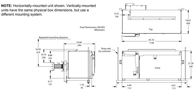
**NOTE:** Bolt-on units can be used only on plug-in busway (800–4000 A—except 800 A copper I-LINE II) with the same number of poles (e.g., do not use 3-pole unit on 3Ø4W busway, or 3Ø4W unit on 3-pole busway).
