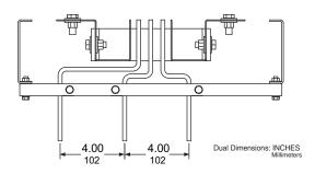
Qwik flanges and closing plates are typically shipped with the switchboard/switchgear. The Qwik flange closing plate closes the gap between the busway and the top of the gear. If a separate Qwik flange or closing plate kit is needed, the catalog numbers can be created by adding the suffix "QF" or "CP" respectively to the prefix of the busway being installed. For example: AF2530GQF or CF2312GCP.
