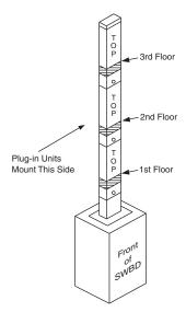
Figure 2: Plug-In Riser Fed by Switchboard
