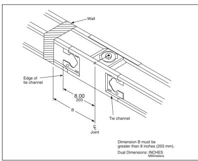
Figure 18: Joint Accessibility Requirements
