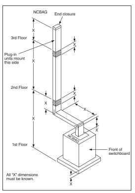
Figure 13: Typical Information Needed for Riser
