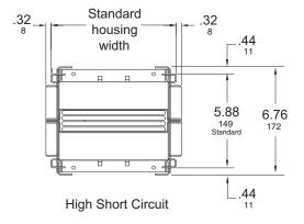
.64 in. (16 mm) wider than standard housing width. .88 in. (22 mm) wider than standard housing height.
