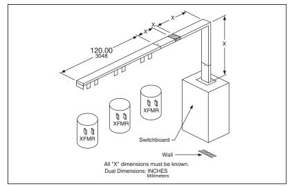
Figure 9: **Transformer Tap for Three Single-phase Transformer**
