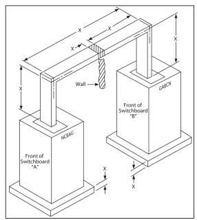
Figure 17: Measurements Needed for Feeder Type Run
