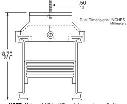
$\ensuremath{\text{NOTE:}}$  Nuts and 1/2 in. (13 mm) drop rods supplied by customer.
