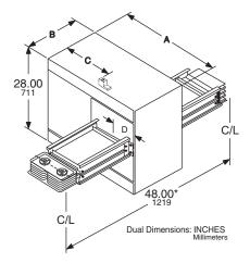
$^{\ast}$  3000 A / 3200 A / 4000 A / 5000 A Center Tap Box Length—60 in. (1524 mm)
