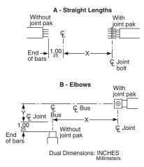
Figure 22: Missing Link Dimensions
