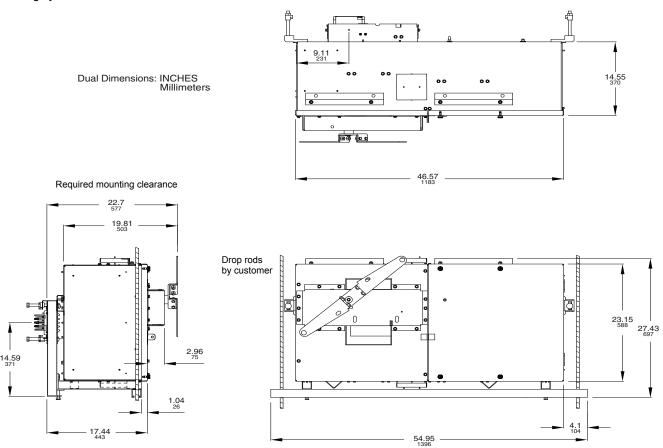
**NOTE**: Bolt-on units to be used only on plug-in busway (800–4000 A—except 800 A copper I-Line II) with the same number of poles (for example, do not use 3-pole unit on 3Ø4W busway).
