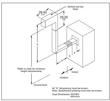
Figure 6: **Typical Vertical Service Head Application**
