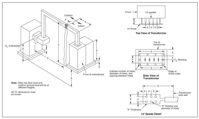
Figure 10: Information Needed for Bussed Transformer Connection (Throat Type)
