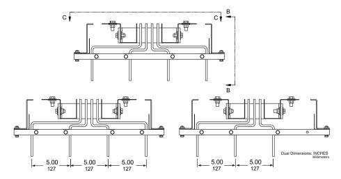
New Qwik flanges and closing plates are typically shipped with the switchboard/switchgear. The new Qwik flange closing plate closes the gap between the busway and the top of the gear. If a separate new Qwik flange or closing plate kit is needed, the catalog numbers can be created by adding the suffix "NQF" or "CP" respectively to the prefix of the busway being installed. For example: AF2530GNQF or AF2530GCP.
