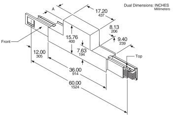
**NOTE:** Expansion joint permits  $\pm$  1.5 in.  $\pm$  38 mm expansion. Use recommended only when busway passes through building expansion joint.
