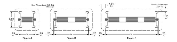
NOTE: Dotted line indicates the profile of the joint covers for Outdoor Feeder busway. The profile for indoor fittings is the same as the busway itself.
