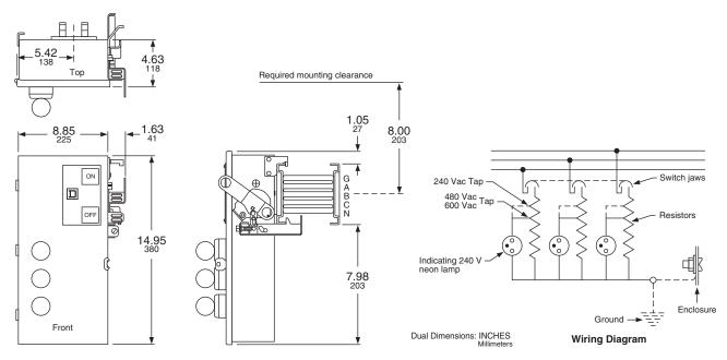
NOTE: The ground detector and neutralizer plug-in unit consists of a disconnect, a high resistance connection from each phase-to-ground, and neon indicating lights wired in parallel with the resistors. The resistors provide a discharge path for high transient voltages that can be impressed temporarily on the busway system.
