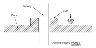
Figure 16: Waterproof Curb Recommended at Floor Opening
