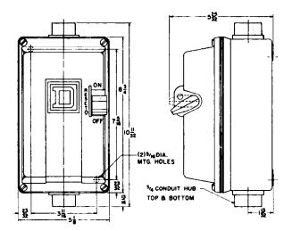
Class 2510 Type M Size M-0 (AC - DC) & M-1 (DC) NEMA Type 4X Watertight, Corrosion-Resistant Glass Polyester Enclosure Approximate Shipping Weight 6 pounds
