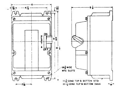
Class 2510 Type M Sizes M-0, M-1, and M-1P NEMA Type 7 & 9 Hazardous Location Cast Iron Enclosure Approximate Shipping Weight 18 pounds
