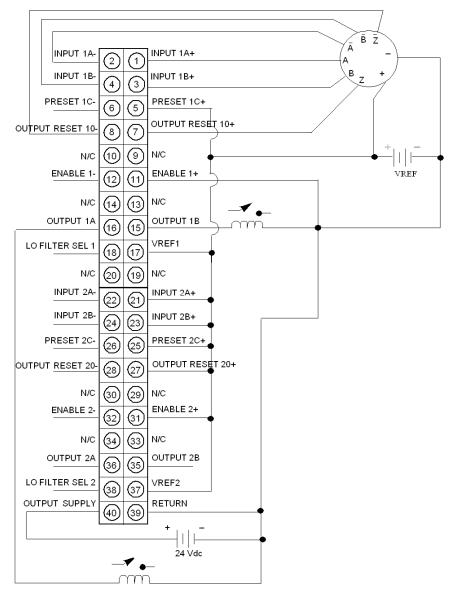
NOTE: Zero pulse resets Output 1A and 1B
