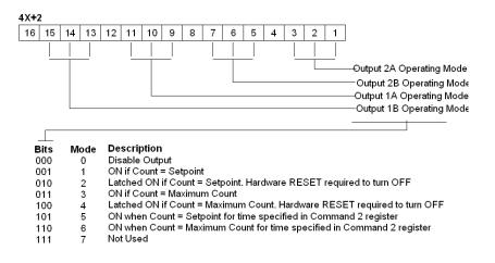
The following figure shows the 4x + 2 output register for command 1.
