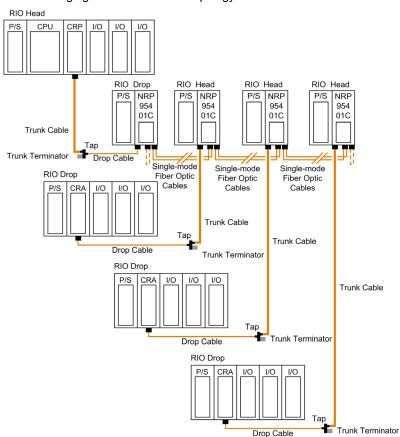
**NOTE:** The total distance between the first and the last fiber optic repeater is limited by the maximum allowable power loss from end-to-end (16 km over 9/125 µm fiber). Power loss includes the fiber optic cable attenuation, connector losses at the fiber optic receiver and transmitter ports, and the system margin of 3 dB.
