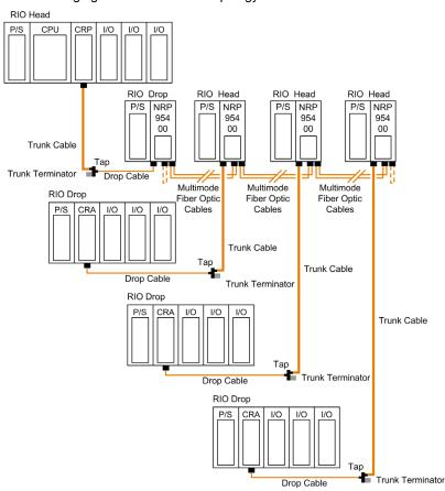
**NOTE:** The distance between nodes on fiber is limited by the maximum allowable power loss from end-to-end (3 km over 62.5  $\mu$ m fiber). Power loss includes the fiber optic cable attenuation, connector losses at the fiber optic receiver and transmitter ports, and the system margin of 3 dB.
