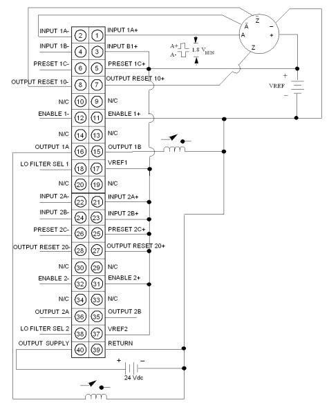
NOTE: Zero pulse resets Output 1A and 1B
