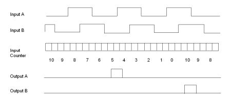
Count is from 10 (Maximum Count) -> 0 Output A turns on at Setpoint = 5 Output B turns on after Input Count = 0 **NOTE:** Outputs are not latched.
