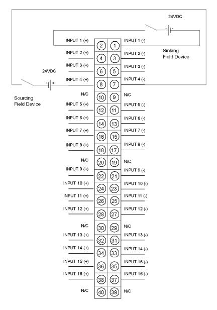
**NOTE:** Either shielded or unshielded signal cables may be used (the user should consider using shielded wire in a noisy environment). Shielded types should have a shield tied to earth ground near the signal ground.
