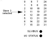
Display of the state of the I/O bits of the selected slave:
