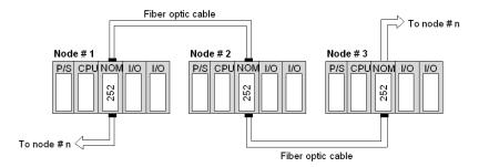
**NOTE:** The distance between nodes on fiber is limited by the maximum allowable power loss from end-to-end (3 km over 62.5 mm fiber). Power loss includes the fiber optic cable attenuation, connector losses at the Fiber Optic Receiver and Transmitter ports, and the system margin of 3 dB.
