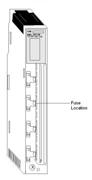
**NOTE:** Turn off power to the module and remove the field wiring terminal strip to gain access to the fuse.
