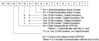
When = 0, if module communication with the bus is lost, outputs are disabled. When = 1, outputs continue to operate as configured.
