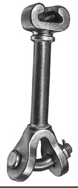
Hot Line Socket Y-Clevis, Ductile Iron, 0.875" Curved Bolt, UTS 50,000 lb; For use with ANSI class 52-8 & 52-11 insulators.
