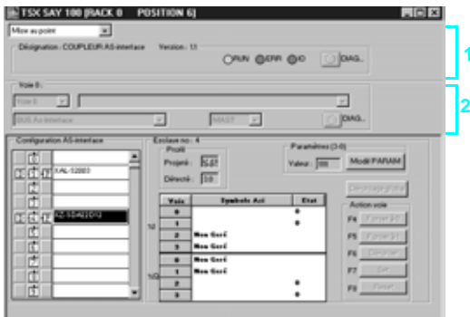
Diagnostics of the TSX SAY 100 module using PL7
