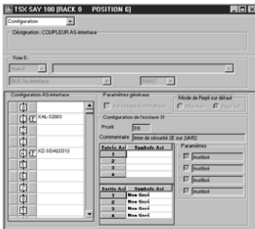
Configuration of slave devices for TSX SAY 100
