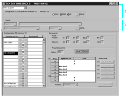
Diagnostics of the TSX SAY 1000 module using PL7
