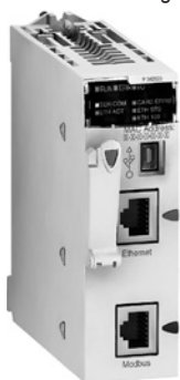
Ethernet port integrated in the CPU (for example with BMXP342020/2030 or Modicon M340 CPU)
