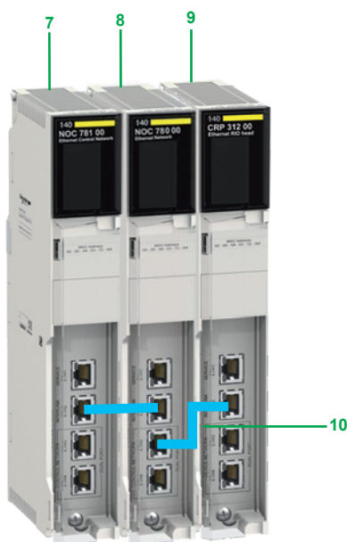
Example of NOC and CRP module combination: 140NOC78100 / 140NOC78000 / 140CRP31200
