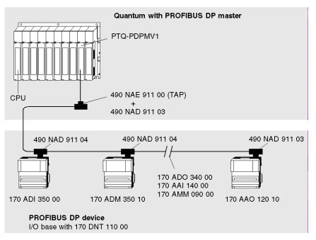
**NOTE:** A PROFIBUS terminating connector (e.g. 490 NAD 911 03) must always be used at the front and back ends of the bus.
