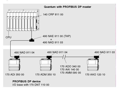
**NOTE:** A PROFIBUS terminating connector (e.g. 490 NAD 911 03) must always be used at the front and back ends of the bus.
