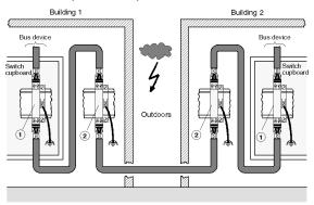
Type and number of lightning conductors made by the firm Dehn und Söhne GmbH &Co KG suitable for a PROFIBUS DP cable
