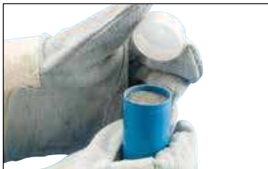
Fig. 20 Next, take the tube of welding material included in the Cadweld Exolon package and remove the lid over the mold crucible.
