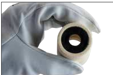
Fig. 6 Each Cadweld Plus One Shot contains a rubber grommet at the bottom of the mold. Place the mold onto the ground rod until the ground rod reaches the wire stopper and cannot go any further.
