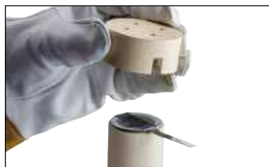
Fig. 10 Place the ceramic lid onto the mold.
