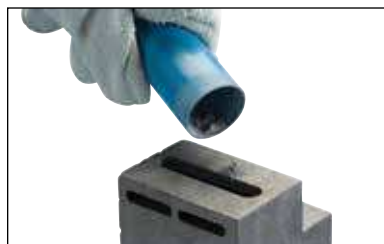
Fig. 23 Close the lid and pour the remaining 3/4 to 2/3 of the starting material into the slot on the mold cover.
