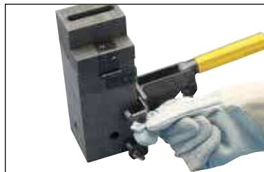
Fig. 7 Tighten the clamp thumbscrews onto the mold.
