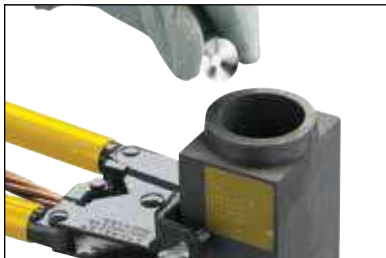
Fig. 18 Insert the steel disk (concave side up) into the mold. Hold the steel disk on the side of the mold and let it slide into place.
