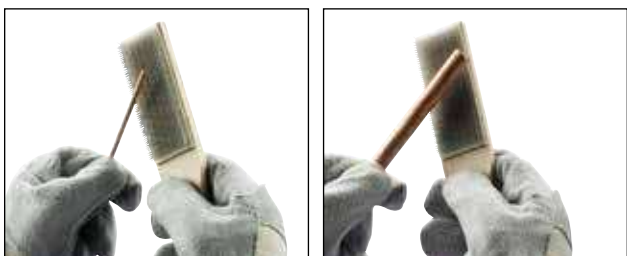
Fig. 5 Next, use a wire brush to further prepare the surface of the conductors and ground rod (nVent ERICO T-313 or T-314 brush). Scrape the outer surface to remove dirt and oxidation. You will notice a slight color change.
