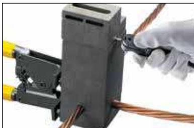
Fig. 18 Place the ignition strip into the control unit connector. Remove or protect fire hazards in close proximity to the connection.
