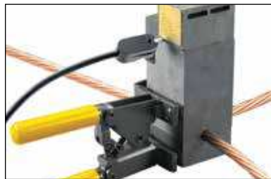
Fig. 19 Close the graphite mold lid. Advise nearby personnel of welding operations in the area.
