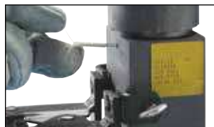
Fig. 23 Next, take an igniter pin and place it halfway into the small hole on the side of the mold, with the loop side facing into the hole. Spread the wire leads.
