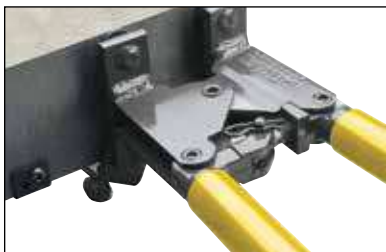
Fig. 9 If the mold does not seal properly, make adjustments to tighten/loosen the handle clamp.
