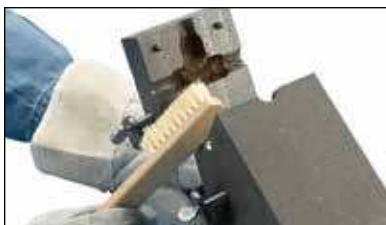
Fig. 27 Cadweld graphite molds will last for approximately 50 connections. Use a soft cotton cloth or a soft bristle brush (nVent ERICO part #T394) to clean inside the mold cavity and cover.
