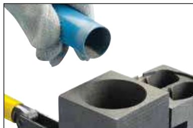
Fig. 22 Pour 1/4 to 1/3 of the starting material over the welding material in the mold crucible.
