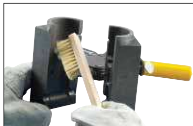
Fig. 30 Cadweld Exolon graphite molds will last for approximately 50 connections. Use a soft cotton cloth or a soft bristle brush (nVent ERICO part #T394) to clean inside the mold cavity and cover; remove any slag left from the exothermic reaction.
