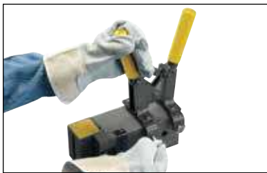
Fig. 7 Tighten the clamp thumbscrews onto the mold.
