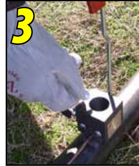
3 Place metal disc in bottom of mold.
