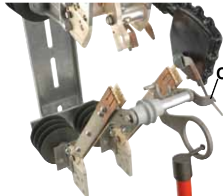
C. Load disconnect blade opens through interrupter.
