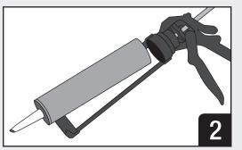
Cartridge: Insert cartridge into cartridge applicator.
