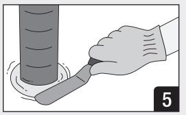
Tool sealant to be flush with substrate.
