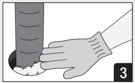
When applicable, install mineral wool to required depth per system specifications.
