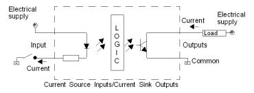
Input side COM field terminal connects to +24V field power supply. Output side COM field terminal connects to the "-" terminal or common of the field power supply.
