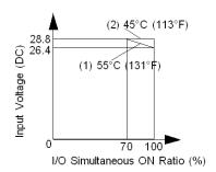
Also, when using the above-mentioned bases at 45° C (113° F), all I/O can be turned on simultaneously at input voltage 28.8 VDC as indicated by line (2).
