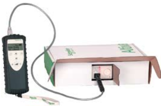
Configuring an Altivar 32 in its packaging: VW3 A8 121 + VW3 A8 126 cordset
