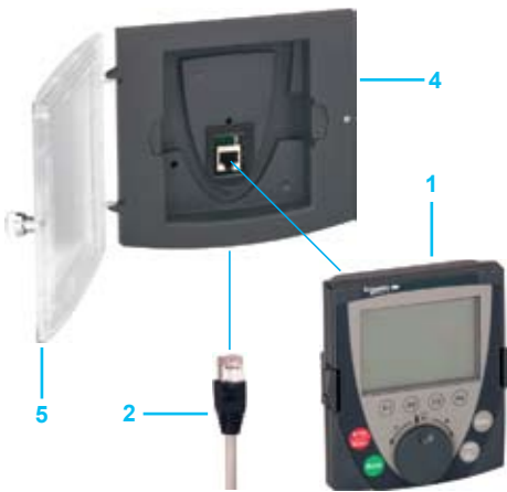
Using the graphic terminal on enclosure door: 1 + 2 + 4 (+ 5, for IP 65)
