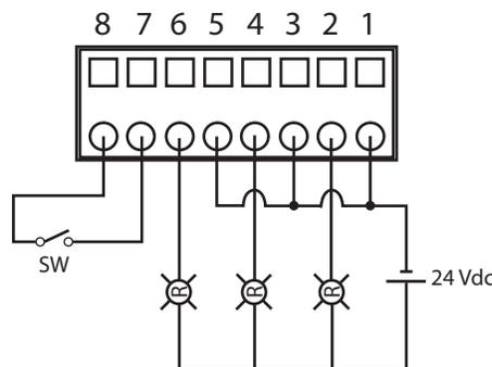
To enable the UPS, close the switch that is connected to the Dry I/O terminals 7 and 8.
