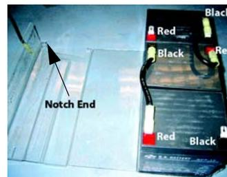
3. Connect the red wire of the harness to the positive terminal (top red) and the black wire of the harness to the negative terminal (bottom black). See photo below for details.
