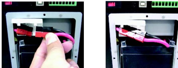
6. To complete the battery installation, close the white connector retainer and reattach the battery door with the three screws (torque of 8.7+/-1.7 lb-in).
