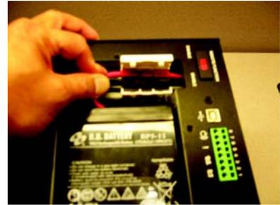
5. To complete the battery installation, close the white connector retainer and reattach the battery door with the three screws (torque of 8.7+/-1.7 lb-in).
