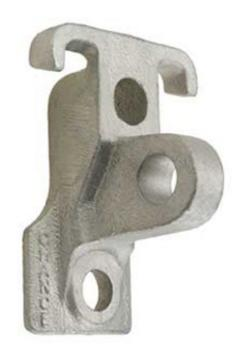
Combination Pole Eye Plate, cast ducile iron. Design traps looped guy between pole and guy plate. Has 13/16" eye hole for guy strain insulator.
