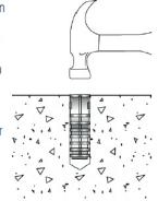
Position fixture, insert the lag bolt, and tighten. The lag bolt length selected should fully engage the entire anchor body.
