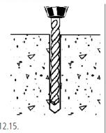
Blow the hole clean of dust and other material. Insert the anchor into the hole until it is flush with the surface. If installing in a mortar joint, position the anchor to expand against the block or brick.
