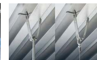
Threaded rod/chain/wire from trapezoidal steel decking
