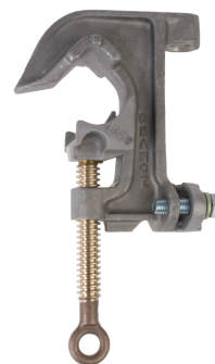
T6000658 Aluminum body, Smooth jaws, Bronze eyescrew with Acme threads, Drilled for 5/8-11 UNC threaded ferrule or T6000311 Tapped for 5/8-11 UNC threaded ferrule
