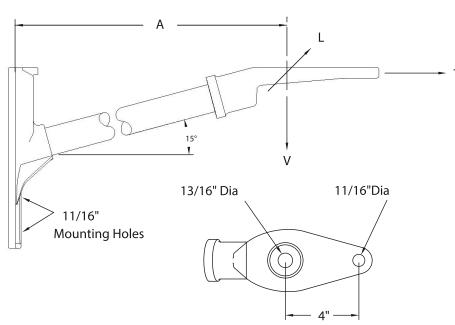
• Base and End Fitting are hot-dipgalvanized ductile iron.
