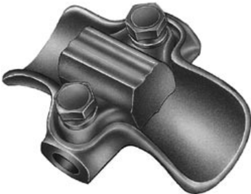
Suspension Clamp, Ductile Iron / Aluminum, Trunnion Style, for use with conductors 0.316 - 0.563
