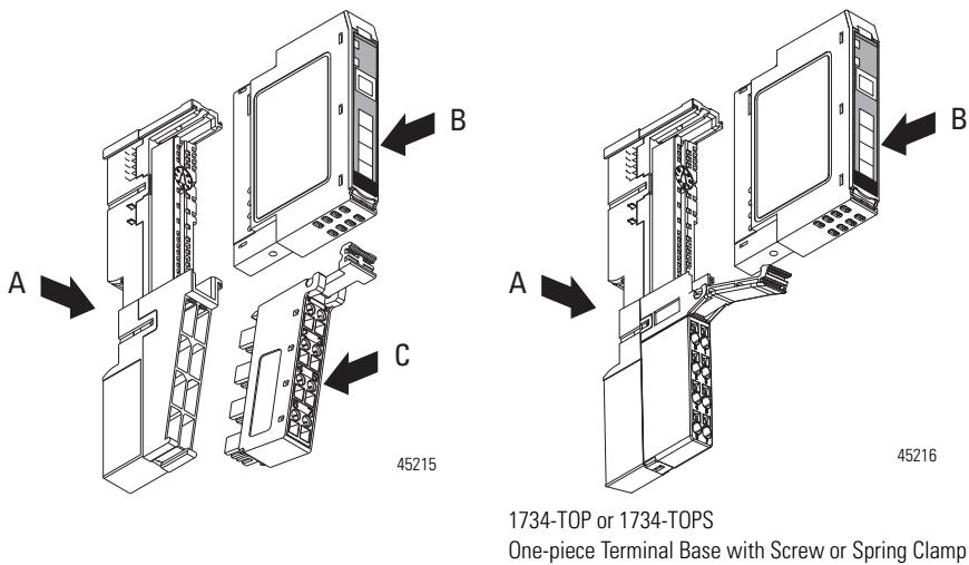
The base (A) mounts onto the DIN rail and provides the backplane. The POINT I/O module (B) snaps into the base. The removable terminal block (C) also snaps into the base and provides the wiring and terminations for field-side connections, as well as system power for the backplane.
