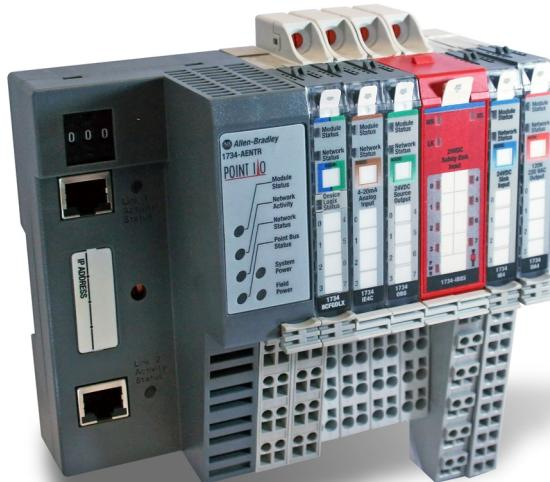
Each POINT I/O module mounts adjacent to the network adapter or another I/O module and removable terminal block (RTB) to connect all field-side wiring. The RTBs are part of the terminal base assembly. They are not included with the I/O modules and must be ordered separately.
