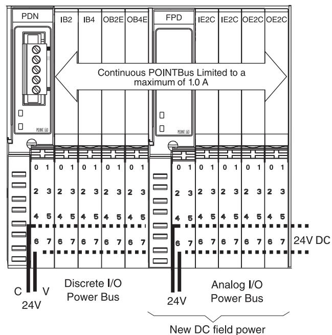
**Wiring Using a 1734-FPD to Create a New DC Device Power Bus**
