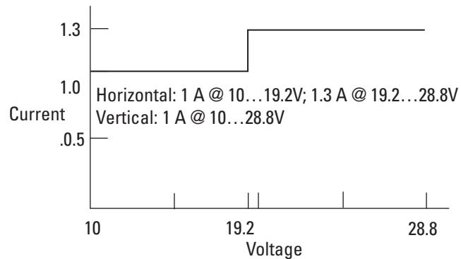
**1734-EPAC Current Derating for Mounting**
