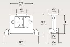
For mounting over doorways with low-ceiling heights, the HCX boasts one of the lowest housing profiles available.
