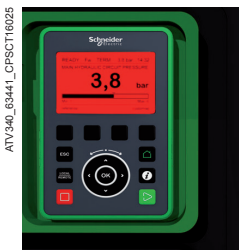
Detected fault: The screen's red backlight is activated automatically
