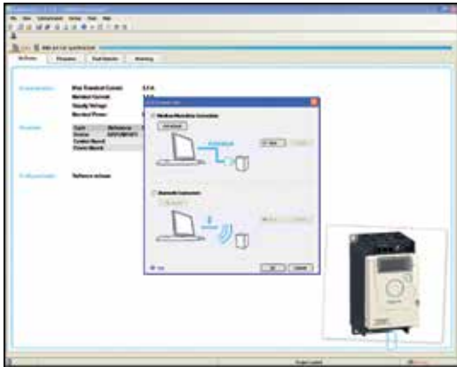
Example of connecting SoMove software to an ATV 12 drive
