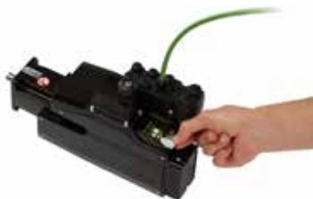
Duplicating an application using the VW3M8705 memory card
