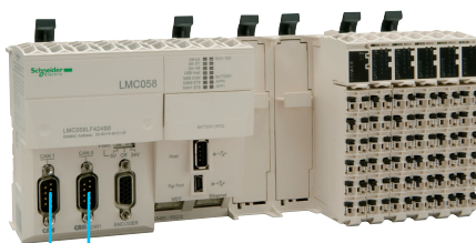
9-way male SUB-D CANopen connector, marked CAN0, for connecting to CANopen bus 9-way male SUB-D CANopen connector, marked CAN1, for connecting to CANmotion bus
