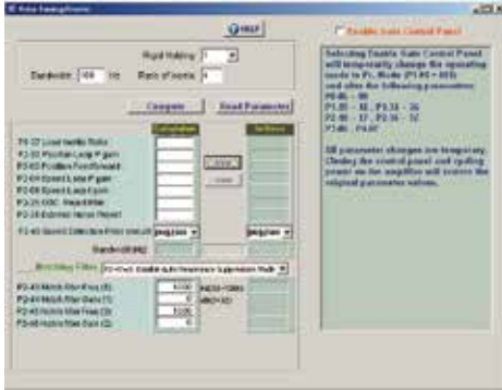
Commissioning using Lexium 23 CT PC software
