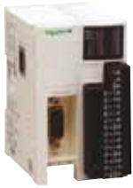
OTB1C0DM9LP CANopen bus interface module
