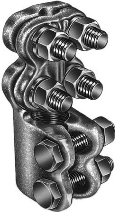
Stud Connector, Bronze, 1-1/8-12 Stud to 0.204-0.575 Cable, Straight
