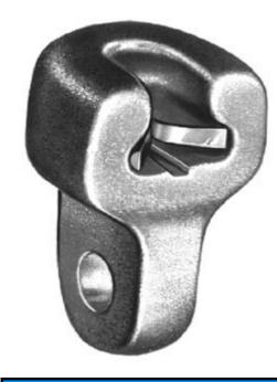
Socket Eye, Ductile Iron, Eye: 1.125" with 0.688" Hole, UTS 30,000 lb; For use with ANSI class 52-3 & 52-5 insulators.
