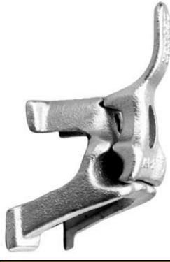
Aerial Suspension Clamp, used to secure messenger to pole face. 5/8" hole in clamp base is tapped to remain in position when clamp half is removed. Top hook supports cable during installation.
