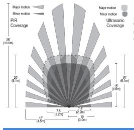
For best performance, Wattstopper recommends using this sensor in spaces no larger than 18' x 15'.
