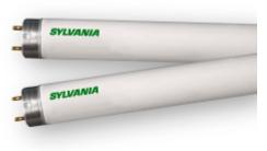
General48" MOL, T8 OCTRON XP Extended Performance, Longer Life, 4100K colorDescription:temperature rare earth phosphor, 85 CRI, ECOLOGIC 3, suitable for operation<br/>on IS or RS ballast
