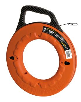
High strength spring steel fish tapes are stiff for long runs and are great for heavy duty wire pulls. Permanent, laser etched 1' (0.3 m) increments on the tape allow you to more accurately measure the depth of conduit runs and determine the amount of tape left to pay out. Polypropylene case and handle are extremely durable and offer the maximum in shock and impact resistance. Raised finger grips help transfer 100-Percent of the winding power from your hand and fingers.
