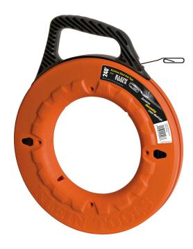
High strength spring steel fish tapes are stiff for long runs and are great for heavy duty wire pulls. Permanent, laser etched 1-foot (0.3 m) increments on the tape allow you to more accurately measure the depth of conduit runs and determine the amount of tape left to pay out. Polypropylene case and handle are extremely durable and offer the maximum in shock and impact resistance. Raised finger grips help transfer 100-Percent of the winding power from your hand and fingers.
