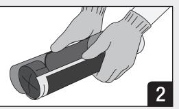
Remove the foam end plugs and set aside. If retrofitting around inplace cables, open the hinged PTD, capture the cables and close the PTD around them.
