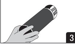
Fit the PTD through the wall/floor and position so that it projects equally from each face.
