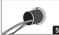
Fit the clamping flange around the PTD, press it flush against the wall/floor, and secure using the supplied mechanical fasteners.
