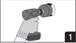
The opening size should be the unit diameter plus 5mm for circular units and overall size plus 5mm for square units.
