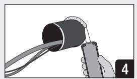
Seal the gap between the PTD and the opening with the appropriate  $3M^{\text{TM}}$  Fire Barrier product (e.g., IC 15WB+, Mortar).
