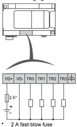
Fast output wiring for TR0... TR3:
