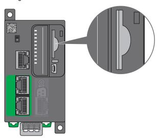
It is possible to set the Write-Control Tab to prevent write operations to the SD card. Push the tab up, as shown in the example on the right-hand side, to release the lock and enable writing to the SD card. Before using an SD card, read the manufacturer's instructions.
