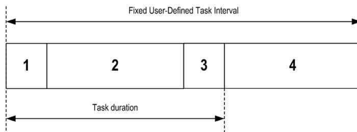
1. **Read Inputs:** The physical input states are written to the %I input memory variables and other system operations are executed.
