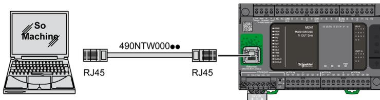
To connect the controller to the PC, do the following:
