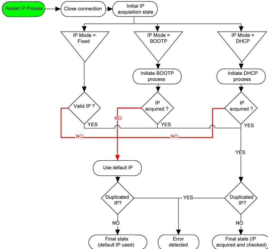
**NOTE:** If a device programmed to use the DHCP or BOOTP addressing methods is unable to contact its respective server, the controller uses the default IP address. It will, however, constantly repeat its request.
