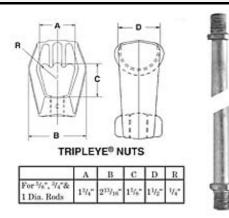
Pisa anchor rod 0.625" (15.9 mm) diameter, 3' 6" (1067 mm) long with Tripleye
