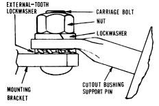
To attach electrical leads, first loosen top and bottom terminal washer faced nuts. Wire brush conductors and apply a coating of oxidation inhibitor before inserting conductor into terminal. Tighten washer faced nuts to approximately 20 ft./lb.
