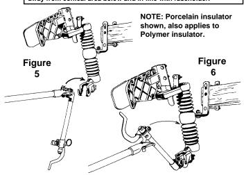
After positioning himself well clear from the vented end and exhaust path of the cutout, the operator should place the disconnect stick in the ring on the upper ferrule of the fuseholder. Rotate the fuseholder to an intermediate position as in Figure 6. Look away from the cutout. Quickly and firmly drive the fuseholder into the closed position. Remove disconnect stick from the ring carefully to avoid opening the fuseholder.
