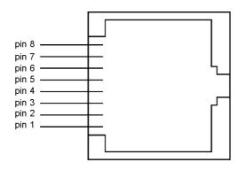
pins 3 and 6 provide pair 1 pins 1 and 2 provide pair 2 remaining pins are not used
