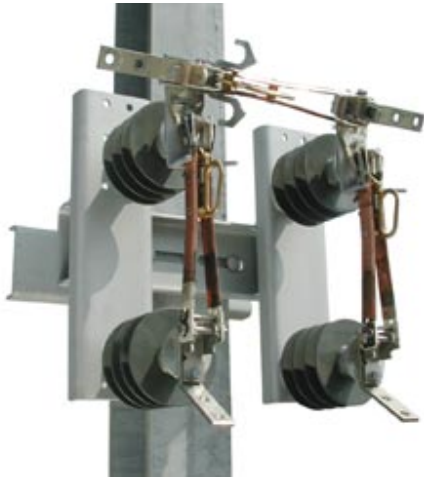
Righthand Opening, 14.4kV, 110kV LIW, 600A By-Pass Switch with Backstrap.
