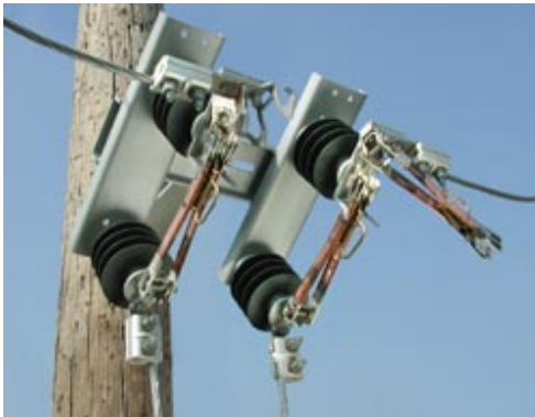
Righthand Opening, 14.4kV, 110kV LIW, 600A By-Pass Switch with Pole Mounting Bracket.
