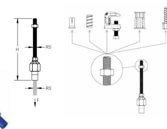
Material: Steel Finish: Electrogalvanized Static Load Safety Factor: 3.5:1
