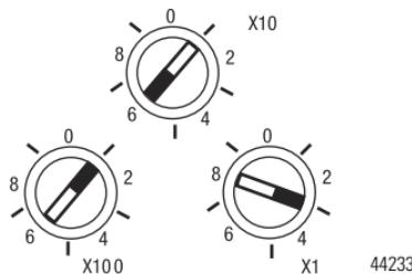
When the switches are set to a valid number, the I/O block's IP address is 192.168.1.xxx (where xxx represents the number set on the switches). The I/O block's subnet mask is 255.255.255.0 and the gateway address is set to 0.0.0.0. When the I/O block uses the network address set on the switches, the I/O block does not have a host name assigned to it or use any Domain Name Server.
