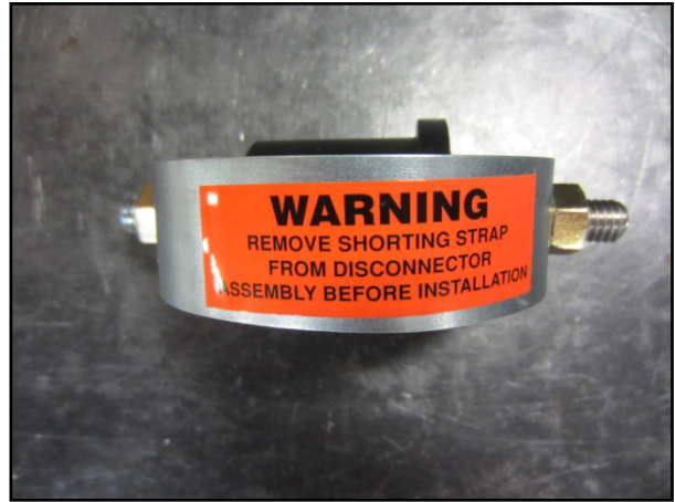
Figure 2: Typical view of Protecta*Lite disconnecter as received.
